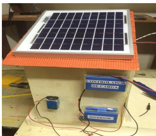
Figur 1. Photovoltaic didactic system: Cell, inverser, charge control and batery.
